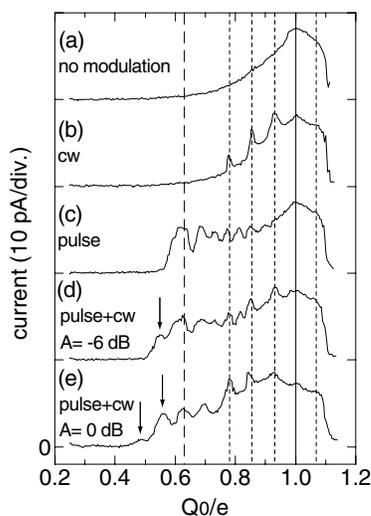
FIG. 2. Current through the probe junction as a function of  $Q_0$ : (a) without microwave or pulse irradiation, (b) with microwave, (c) with pulse, and (d),(e) with both microwave and pulse. Microwave frequency  $f$  is 20 GHz. Pulse length  $\Delta t$  and repetition time  $T_r$  are 80 ps and 64 ns.
