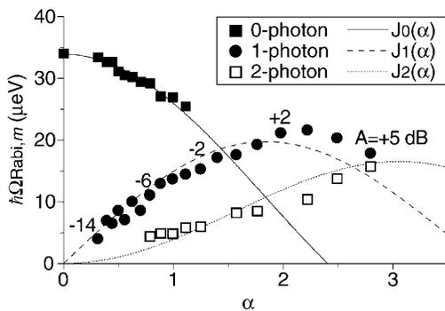
FIG. 4. Rabi-oscillation frequency  $\Omega_{\text{Rabi},m}$  ( $m = 0, 1$ , and  $2$ , respectively, for 0-, 1-, and 2-photon processes) as a function of irradiated microwave amplitude. Lines are the first-kind Bessel functions of the corresponding order,  $J_m(\alpha)$ , where  $\alpha \equiv (2eV_{\text{ac}}/hf)(C_p/C_\Sigma)$ .
