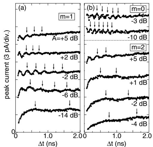
FIG. 3.  $m$ -photon Rabi oscillations observed in the relevant peak current in  $I-Q_0$  curves [see Figs. 2(d) and 2(e)] as a function of pulse length  $\Delta t$ . (a) for  $m = 1$  and (b) for  $m = 0$  and 2. The arrows indicate the period of the oscillations. Each result for different microwave power  $A$  is shifted vertically by 3 pA for clarity.
