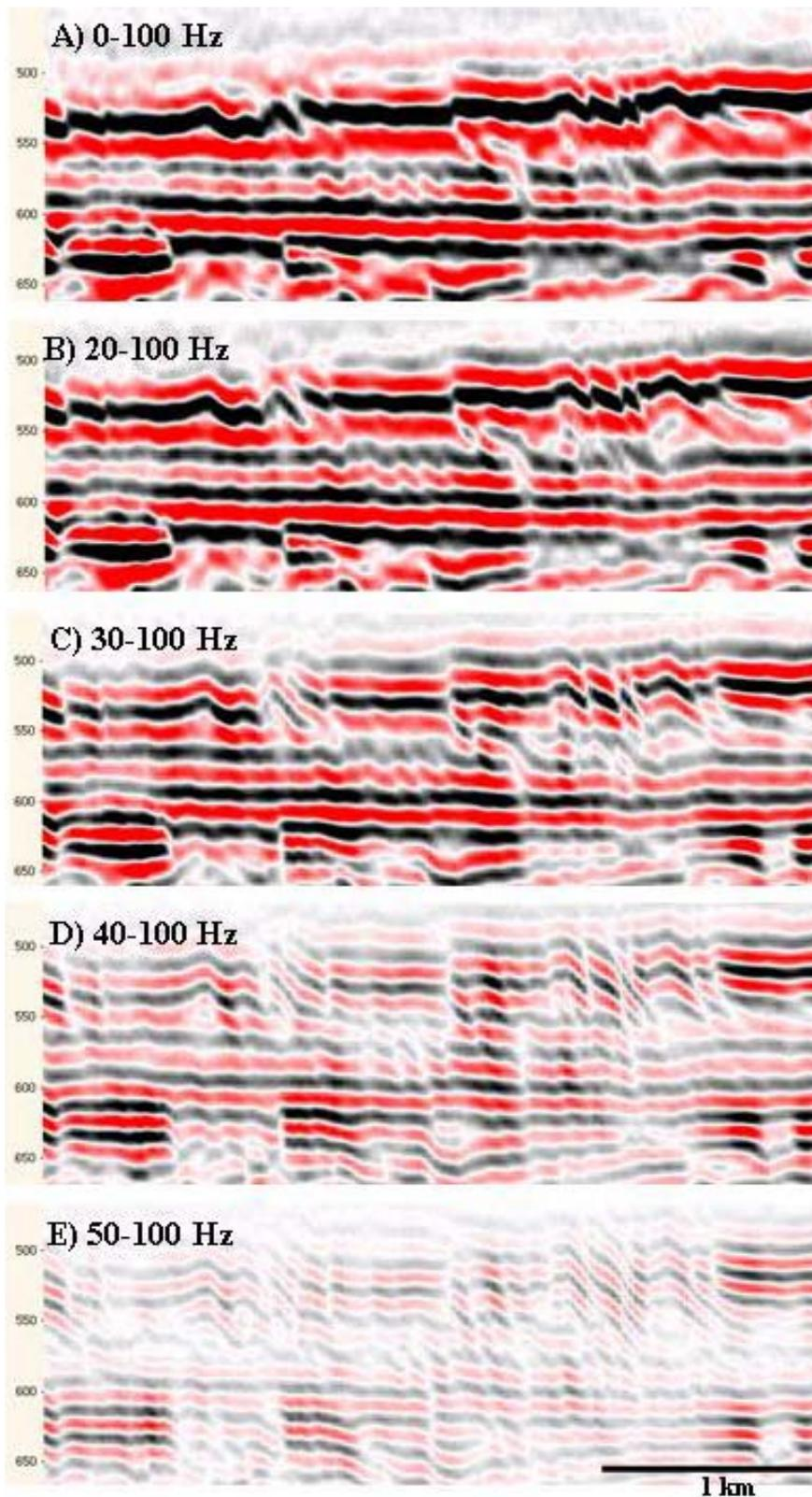
**Figure 3. A-E)** Examples of how a gradual removal (from top to bottom) of the low frequencies in the data apparently enhances the resolution and weakens the amplitude. Features that in A may look like disturbances in the upper part of the succession are in fact thrust sediment sheets stacked in an imbricating manner (D and E). On the left the depth is shown in millisecond two-way travel-time.
