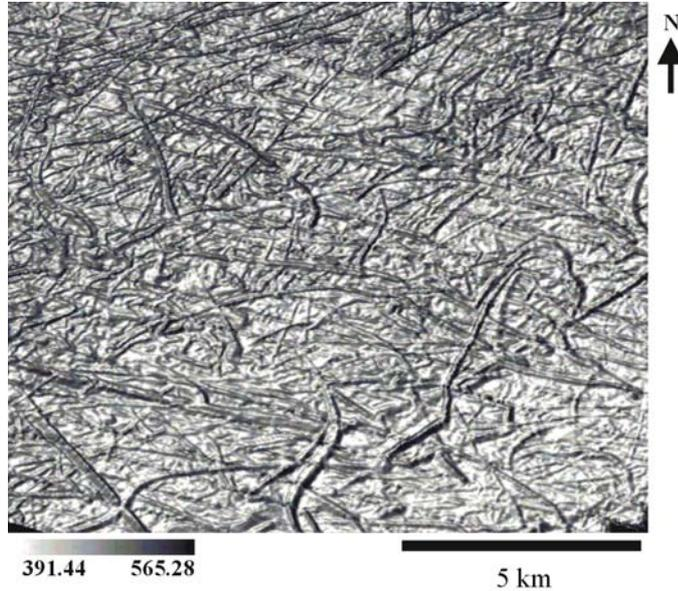
**Figure 2.** Plough mark with a relief from 2,5-20 m, shown on the sea floor from a 3-D survey in the south-western Barents Sea. The scale in the lower left corner indicates depth in milliseconds two-way travel-time. Modified from Rafaelsen et al. (2002).
