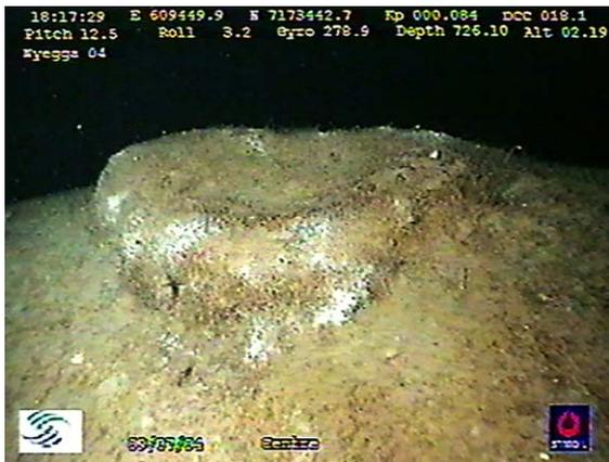
Fig. 3. Video-grabbed image of pingo at location “Ice1” (see ‘1’ in Fig. 2B). The pingo measures about 1 m across, and has rims that protrude about 25 cm out of the seafloor. These rims are partly coated in thin bacterial mats, indicating active seepage. The pingo has a central sag, indicating sub-surface dissolution of hydrates. Note that it is located on top of a dome-shaped portion of the seabed.
