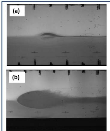
Figure 2. Representative ISW bulge waves; (a) intermediate large-amplitude,  $a_b/h = 1.96$ ; (b) very large-amplitude,  $a_b/h = 5.92$ .
