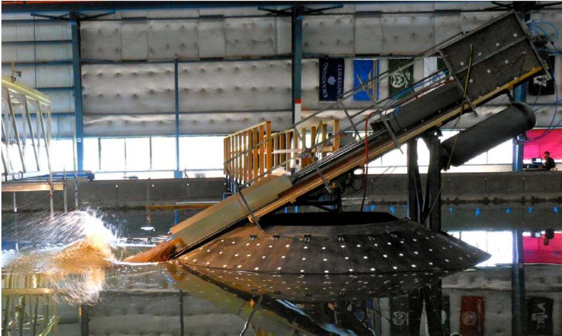
Figure 2. Conical Island setup with tsunami generation by granular landslide impact at  $h = 1.2$  m.
