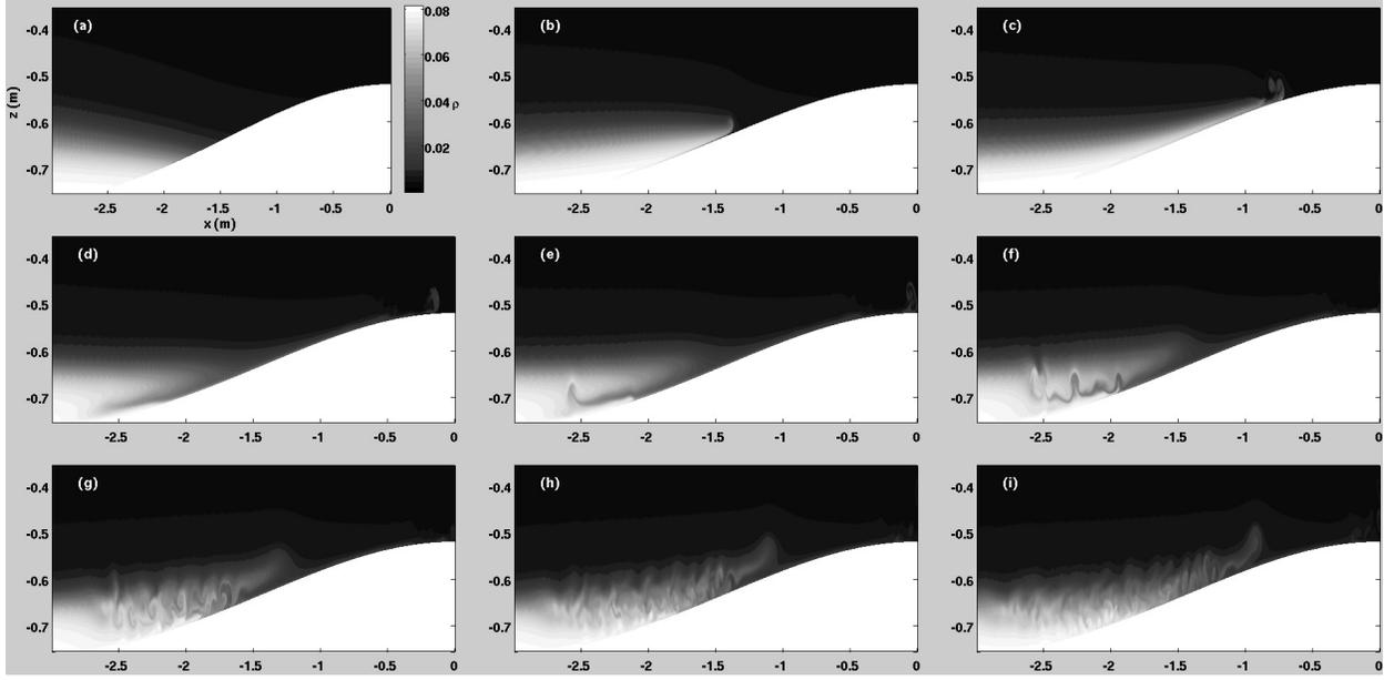
Figure 1: Evolution of experimental-scale shoaling internal seiche.
