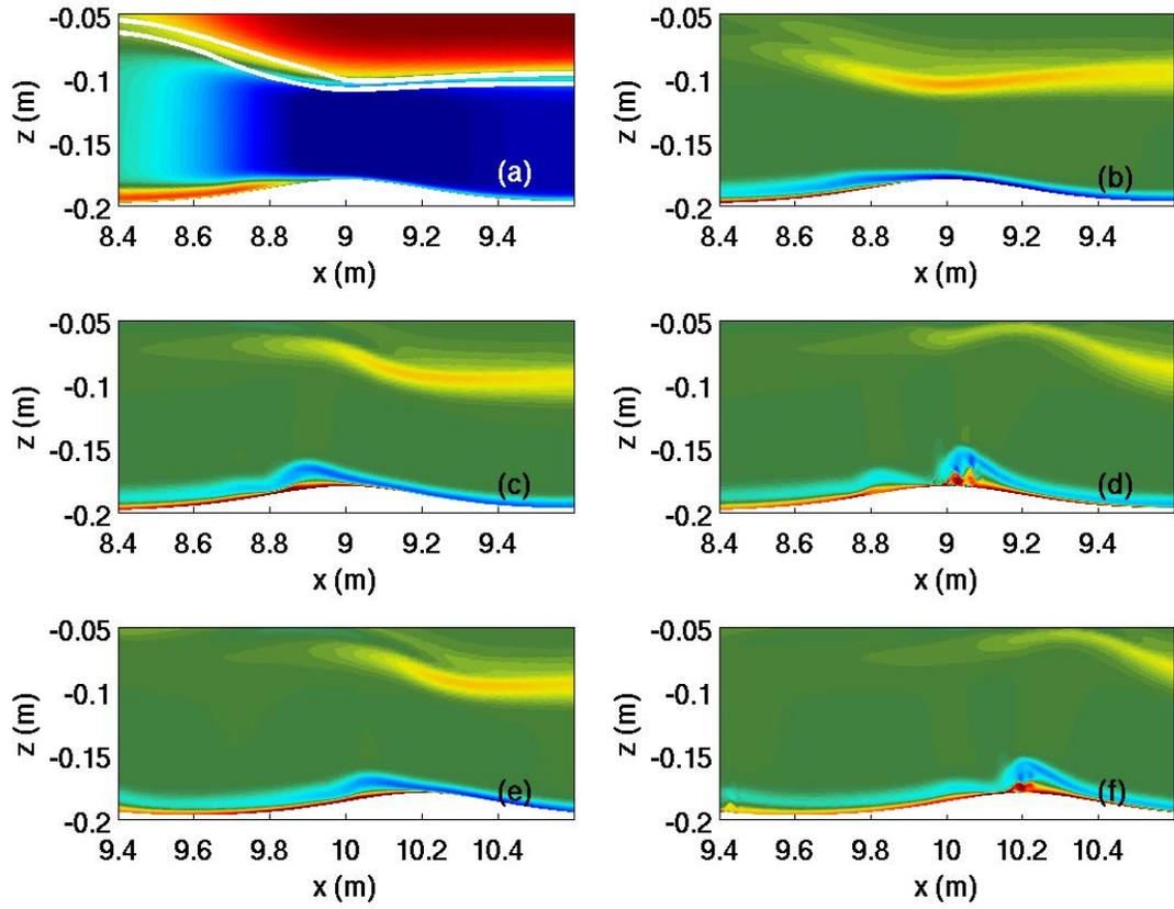
Figure 2: Instability of the prograde jet behind an ISW of depression. (a)  $u$ , (b-f)  $\omega = u_z - w_x$ .
