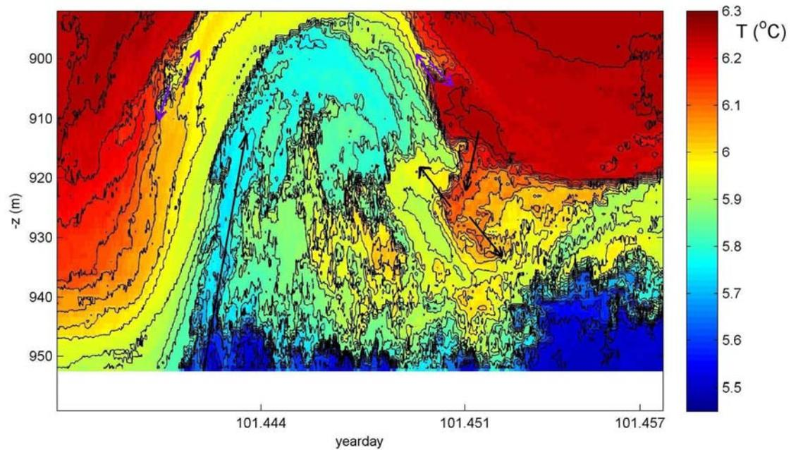
*Time-depth image of 1800 s horizontally by 67 m vertically. It details a large backwards breaking internal wave. This was observed using 61 high sampling rate temperature sensors between 7 and 67 m above the bottom at 959 m, above a slope of Opouawe Bank, off New Zealand, Southern Ocean. Contour intervals every 0.04  $^{\circ}\text{C}$  (black).*
