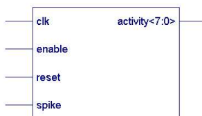
Figure 5.10: Schematic symbol of the activity analyzer module.
