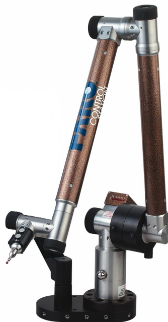
Figure 2.1: Coordinate measuring machine, arm type (FARO).
