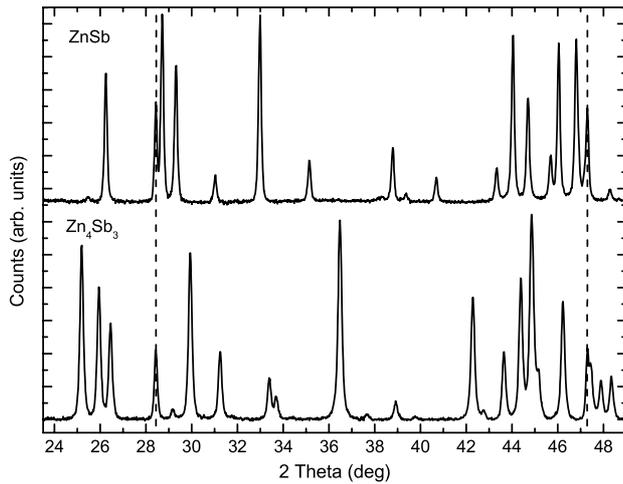
**Figure 1.** Detail of the XRD scan of ZnSb (top) and Zn<sub>4</sub>Sb<sub>3</sub> (bottom). Dashed lines indicate the admixed Si standard.
