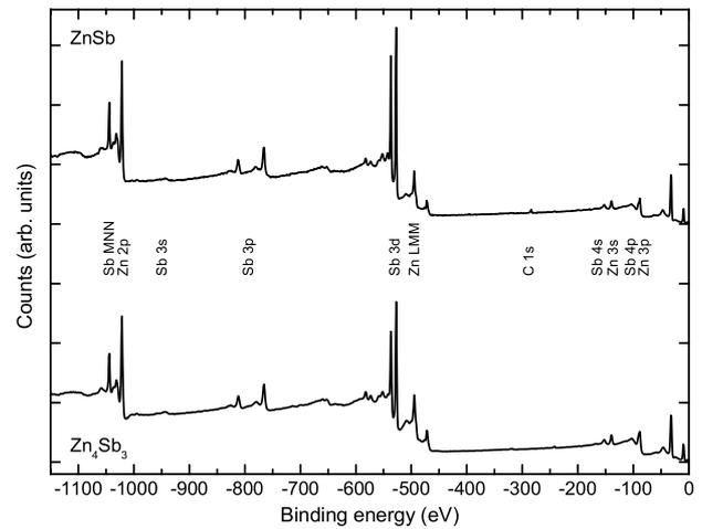
**Figure 2.** XPS survey scan of ZnSb (top) and Zn<sub>4</sub>Sb<sub>3</sub> (bottom). Selected identifying features are labelled.
