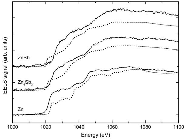
**Figure 4.** EELS spectra (solid lines) and FEFF results (dotted lines) for the Zn  $L_{2,3}$  line in the ZnSb,  $Zn_4Sb_3$  and in pure Zn.
