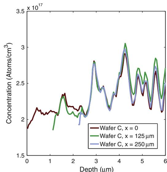
Fig. 3. Li concentration versus depth measured at three different positions ( $x$ ) of wafer C by SIMS. The depth profiles of the second and third crater is shifted by  $1.1 \mu\text{m}$  and  $2.2 \mu\text{m}$ , respectively, as compared with the first crater due to an offset in the cut angle.
