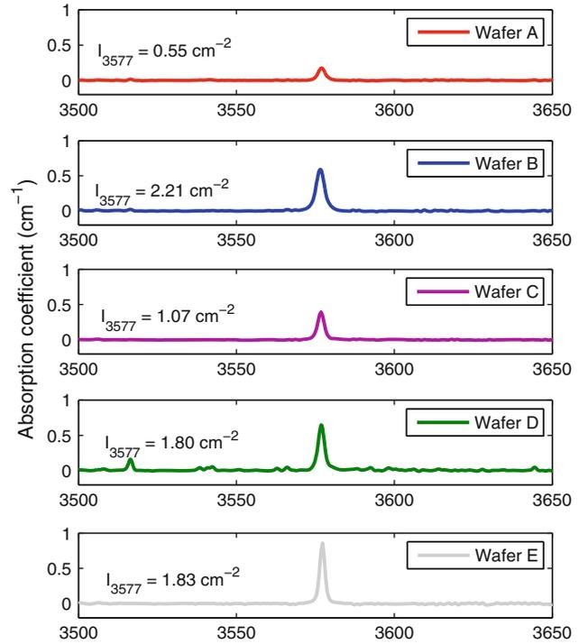
Fig. 1. Infrared absorption spectra measured with light propagating perpendicular to the  $c$ -axis ( $k \perp \vec{c}$ ). The integrated absorption coefficient for the  $3577\text{ cm}^{-1}$  absorption line is shown to vary from wafer to wafer.
