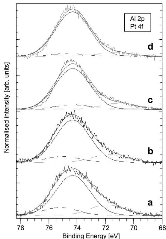
Fig. 10. Al2p peak together with Pt4f doublet in the samples Pt-2 and Pt-1 at 10 Å analysis depth. (a) Pt-2 in reaction mixture, (b) Pt-2 in oxygen, (c) Pt-2 in hydrogen-steam mixture and (d) Pt-1 in reaction mixture, all at 450 °C.
