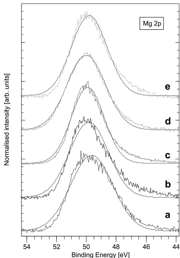
Fig. 7. The Mg2p peak in samples Pt-2, HT and Pt-1 at 10 Å analysis depth. (a) Pt-2 in reaction mixture, (b) Pt-2 in oxygen, (c) Pt-2 in hydrogen-steam mixture, (d) HT in reaction mixture, (e) Pt-1 in reaction mixture, all at 450 °C.
