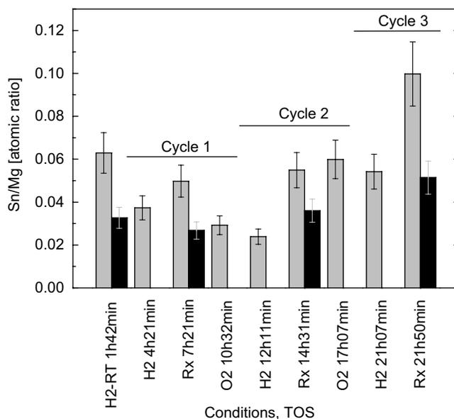
Fig. 11. Sn/Mg atomic ratio in sample Pt,Sn-1 at 10 Å (grey bars) and 14 Å (black bars) analysis depth.
