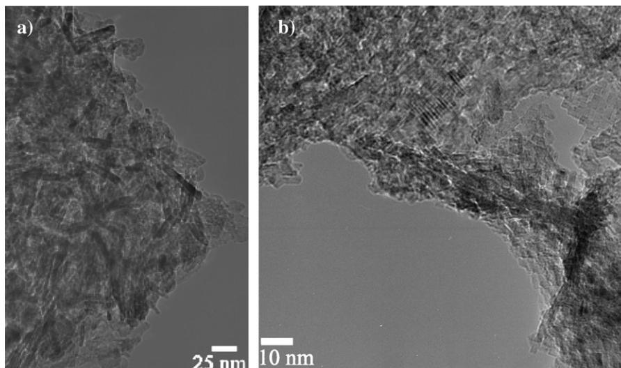
Fig. 1. TEM pictures of (a) Sample HT and (b) Sample Pt-2.
