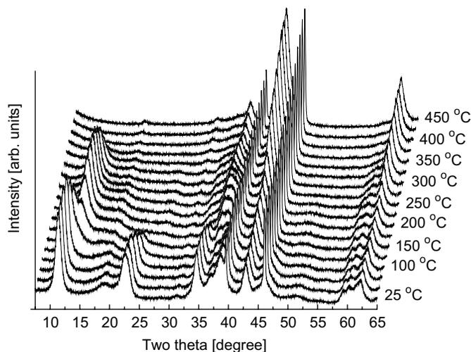
Fig. 2. Temperature resolved XRD-patterns of a Mg(Al)O sample after storage in air for several months, during heating to 450 °C in air. The reflexes at  $2\theta = 39.5^\circ$  and  $46.0^\circ$  are Pt reflexes from the Pt sample holder.
