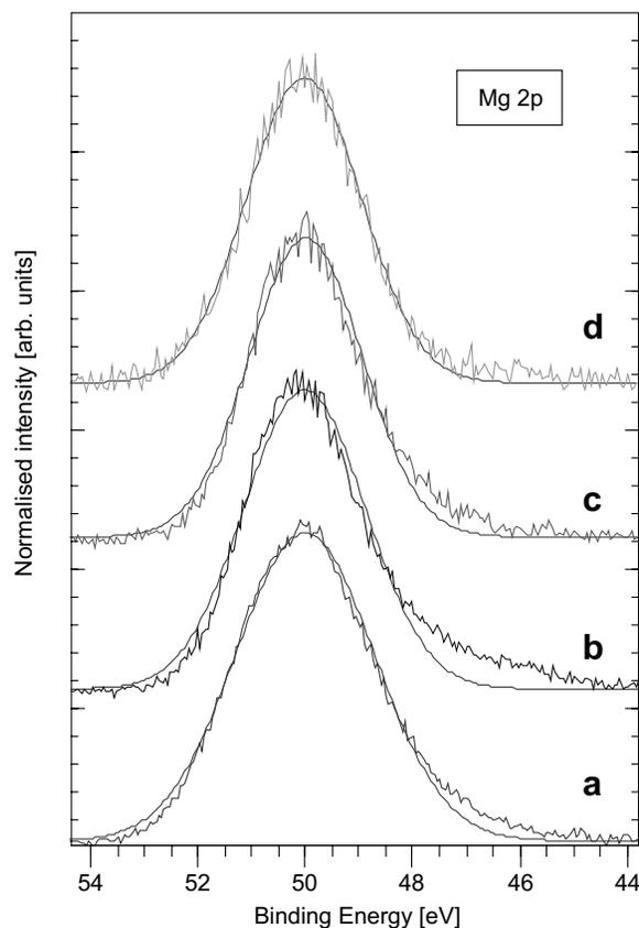
Fig. 6. The Mg2p peak at analysis depth of (a) 10 Å, (b) 14 Å, (c) 17 Å and (d) 21 Å in calcined hydrotalcite (sample HT) under reaction mixture at 450 °C.
