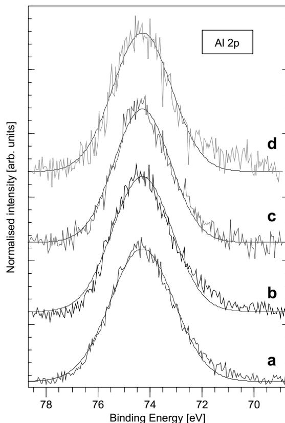
Fig. 8. Al2p peak at analysis depth of (a) 10 Å, (b) 14 Å, (c) 17 Å and (d) 21 Å in sample HT under reaction conditions.
