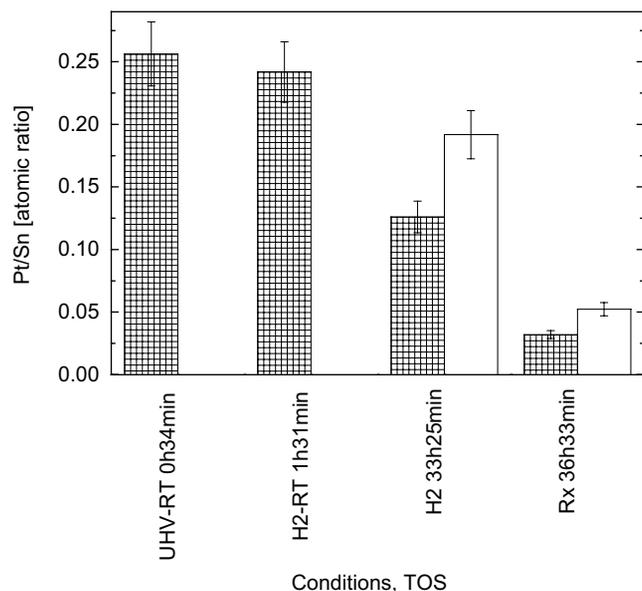
Fig. 14. Pt/Sn atomic ratio in PtSn<sub>2</sub> alloy under different conditions (see Table 1 for details) and at two analysis depths: 8 Å (squared bars) and 15 Å (white bars).
