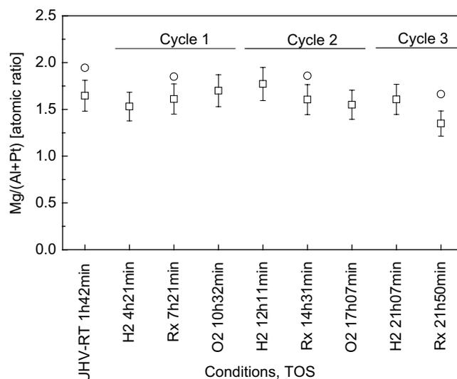
Fig. 13. Mg/(Al + Pt) atomic ratio in sample Pt,Sn-1 at 10 Å (□) and 14 Å (○) analysis depth.
