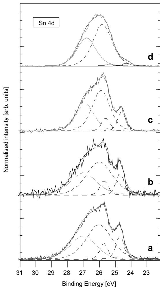
Fig. 16. Deconvolution of Sn4d peak in PtSn<sub>2</sub> alloy at 8 Å analysis depth under following conditions: (a) in UHV at RT, (b) in H<sub>2</sub> at RT, (c) in H<sub>2</sub> at 450 °C and (d) in reaction mixture at 450 °C.
