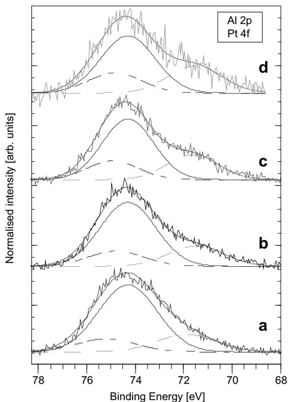
Fig. 9. Al2p peak together with Pt4f doublet in the sample Pt-2 under reaction conditions at analysis depth of (a) 10 Å, (b) 14 Å, (c) 17 Å and (d) 21 Å.
