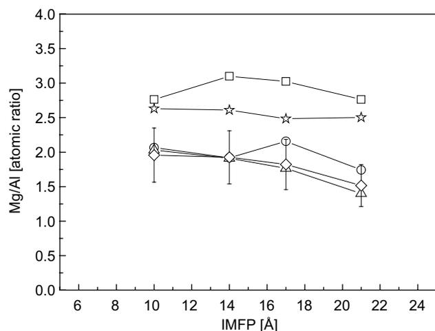
Fig. 5. Mg/Al or Mg/(Al + Pt) atomic ratio in the support material as function of analysis depth. □ Sample HT under reaction conditions, ☆ Sample Pt-1 under reaction conditions, ○ Sample Pt-2 under reaction conditions, △ Sample Pt-2 under oxidation conditions, ◇ Sample Pt-2 in hydrogen–water mixture, all at 450 °C (see Table 1 for details).
