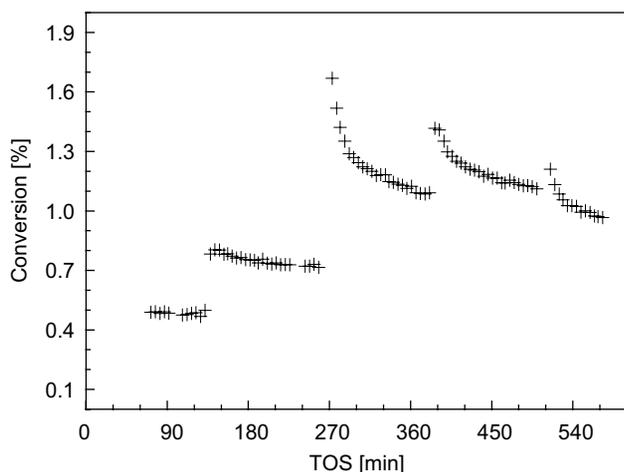
Fig. 3. Activation of sample Pt,Sn-1 in a conventional test reactor at 450 °C. Reaction conditions:  $\text{H}_2:\text{C}_2\text{H}_6:\text{CO}_2:\text{Inert} = 1:1.6:3:4.3:51$ , 450 °C, 1 atm,  $\text{WHSV} = 1.6 \text{ h}^{-1}$ .
