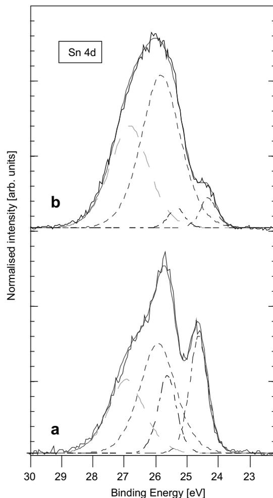
Fig. 17. Deconvolution of Sn4d peak in PtSn<sub>2</sub> alloy at 15 Å analysis depth under following conditions: (a) in H<sub>2</sub> at 450 °C and (b) in reaction mixture at 450 °C.
