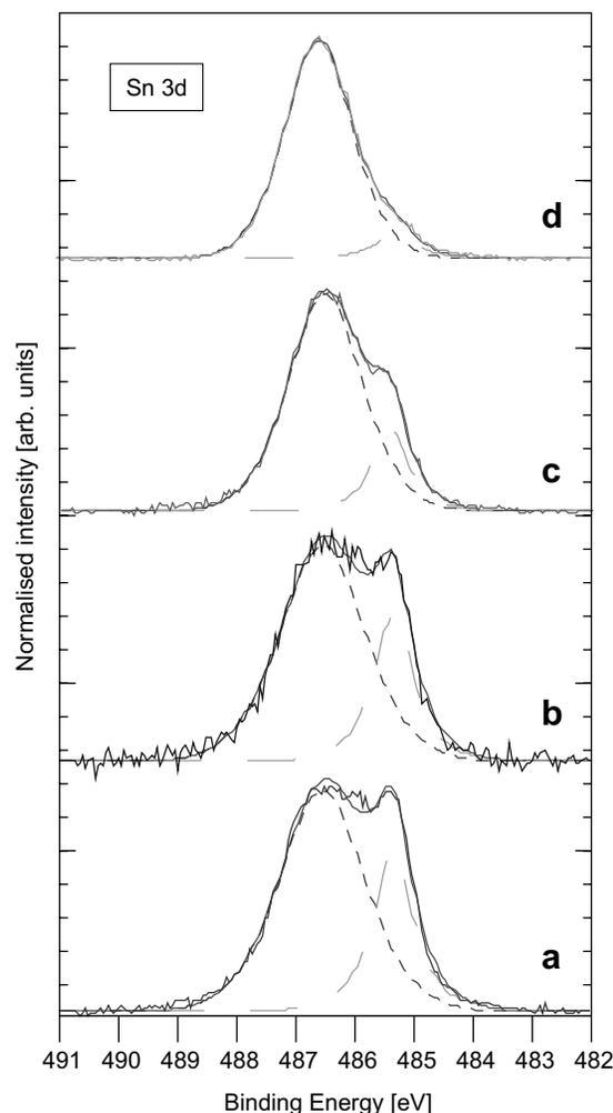
Fig. 15. Deconvolution of Sn 3d peak in PtSn<sub>2</sub> alloy at 8 Å analysis depth under following conditions: (a) in UHV at RT, (b) in H<sub>2</sub> at RT, (c) in H<sub>2</sub> at 450 °C and (d) in reaction mixture at 450 °C.
