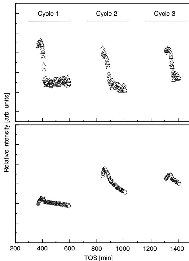
Fig. 4. Activation of sample Pt,Sn-1 during *in situ* XPS measurements under reaction conditions at 450 °C.  $\text{H}_2:\text{C}_2\text{H}_6:\text{H}_2\text{O} = 1:1.5:7.5$ , total pressure 0.3 mbar. Upper curve:  $[(m/e\ 28):(m/e\ 30)]$ , representing ethene production. Lower curve:  $[(m/e\ 44):(m/e\ 30)]$ , representing  $\text{CO}_2$  production.
