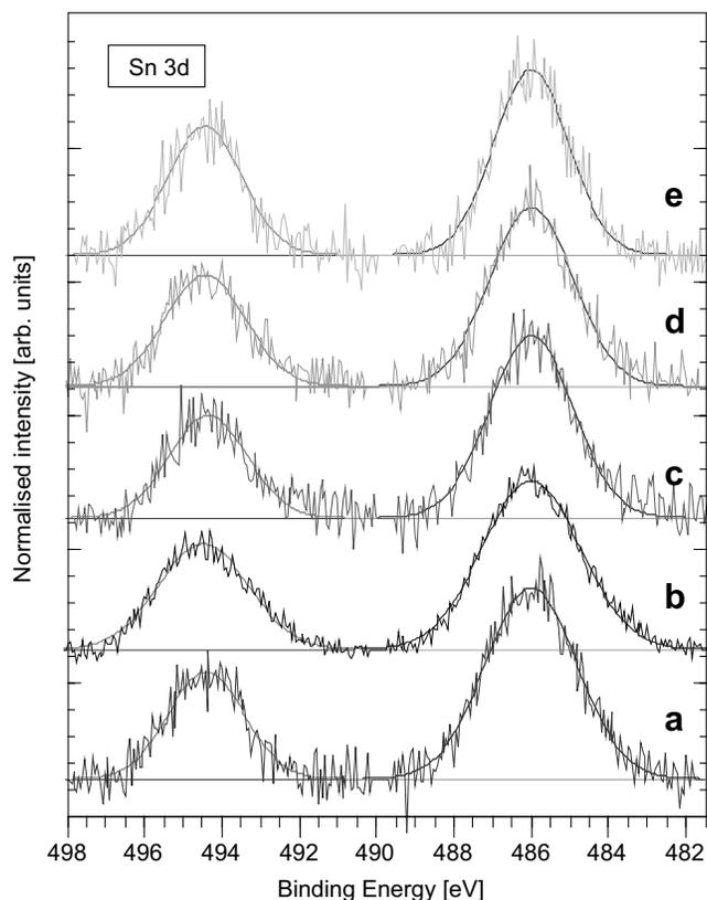
Fig. 12. Sn3d doublet in sample Pt,Sn-1 at two analysis depths and in different gas mixtures, (a) 10 Å, H<sub>2</sub>, room temperature, (b) 10 Å, O<sub>2</sub>, 450 °C, (c) 10 Å, H<sub>2</sub>, 450 °C, (d) 10 Å, reaction mixture, 450 °C and (e) 14 Å, reaction mixture 450 °C.
