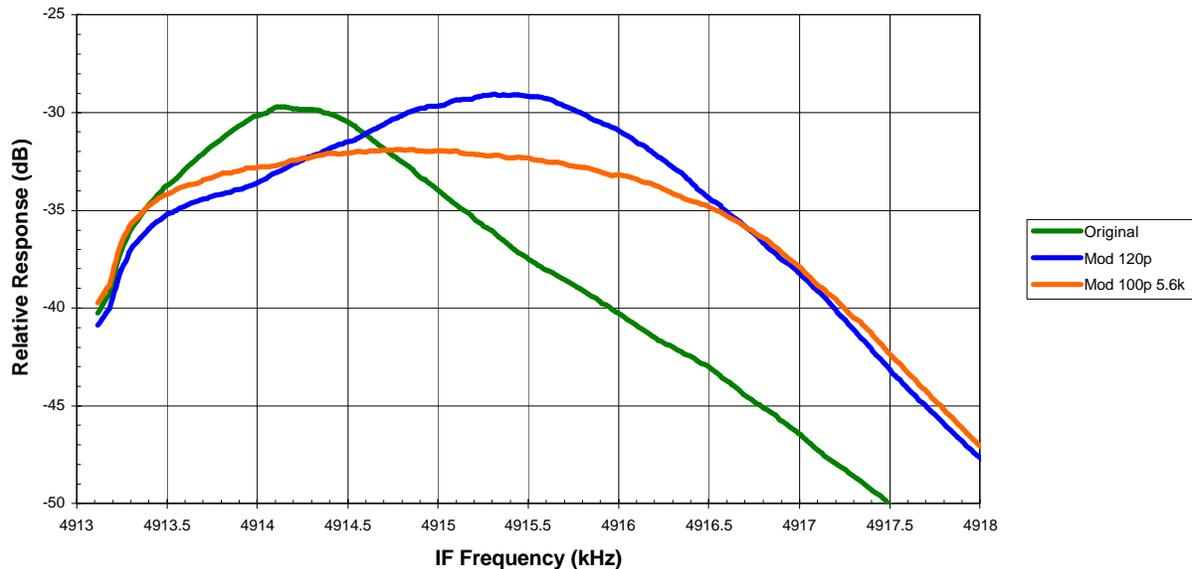
The K2's 2nd Xtal Filter needs to be as flat as possible from 4914 to 4916 kHz with the standard SSB filter. With the wider filters, it may need to remain flat up to 4916.5 kHz. The original design, shown in Green, had a sharp high frequency rolloff with 4916 kHz being 10 dB below the peak response. This resulted in lots of high frequency attenuation in LSB and lots of low frequency attenuation in USB on the bands below 21 MHz.
