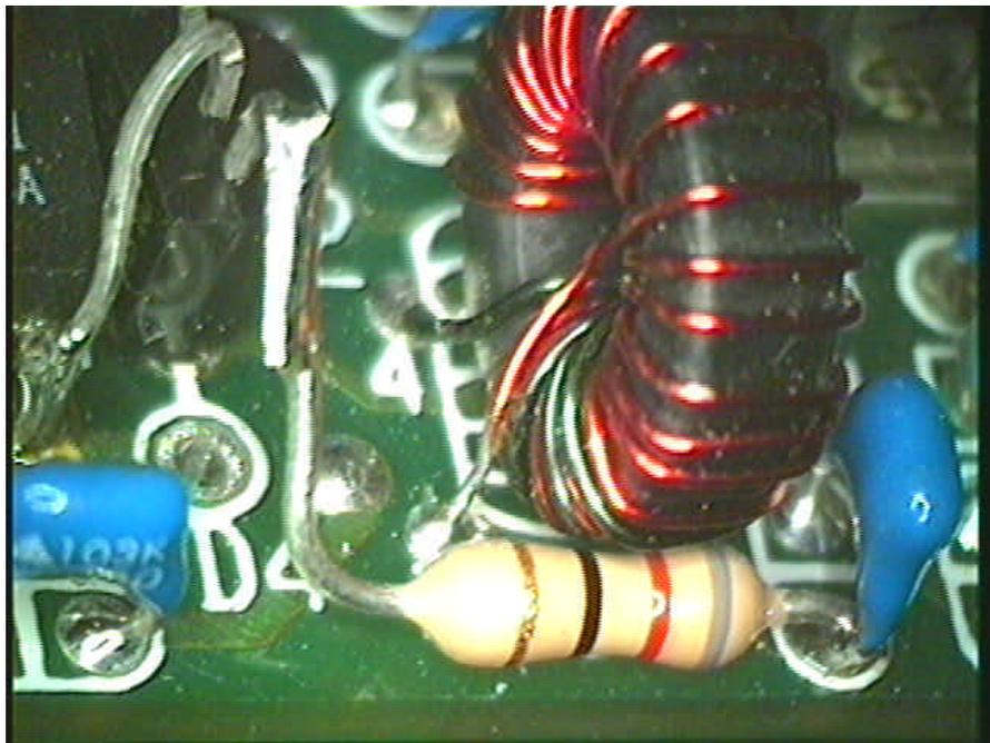
5. On the back side of the PC board, run a 2.7K resistor between Pin 4 of T2 (R6 makes a good connection point) and ground. This resistor limits the reverse bias applied to the B-E junction of the PN2222 to 3 volts and avoids any chance of a base-emitter breakdown.
