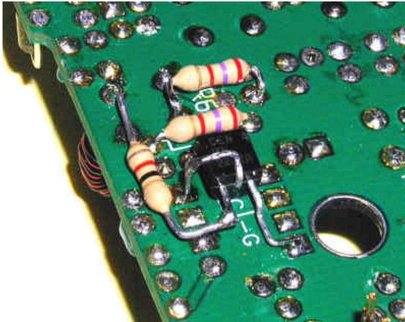
This change has worked well in the two K2's that have been modified using it. It certainly will help anyone who has a low output microphone. Additionally, it provides the increased gain that allows a reduction in the audio drive level at the input of the NE602, which is described in the next section.
