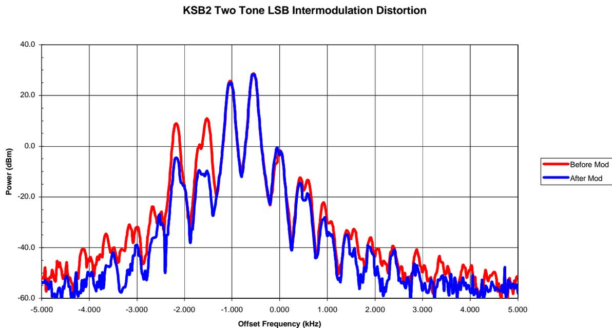
This change should only be done if the KSB2 Increased Gain Modification has also been added. The net results of both changes will be an increased gain in the KSB2 of about 4 dB. This is enough gain to overcome the marginal SSB drive on 10 meters, but may not be enough additional gain for a low output microphone. If your microphone has low output and you cannot get to full power on 10 meters, then you may not want to apply the Reduced Intermodulation Distortion Modification.
